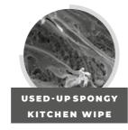
Damaged porous structure with captured dirt
