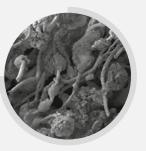
Used sponge - disintegrating Fibre mesh with captured dirt
